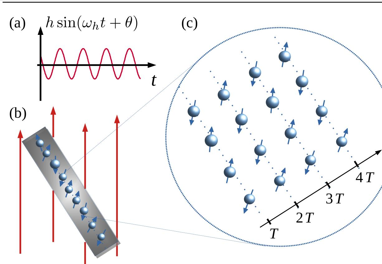
The sensor is described by a Floquet Hamiltonian that can enter a TC phase  $\infty$  $\hat{H}_s = \sum_i \left[ J_i \hat{\sigma}_i^z \hat{\sigma}_{i+1}^z + \sum_{\alpha = x, z} b_i^\alpha \hat{\sigma}_i^\alpha - \frac{\phi}{2} \sum_{n = -\infty}^\infty \delta(t - nT) \hat{\sigma}_i^x \right]$
