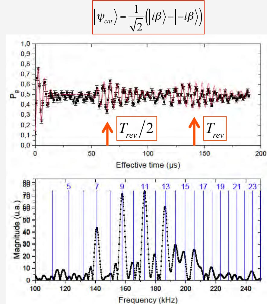
"Odd" cat state: the Rabi oscillation spectrum reveals the **cat parity**
